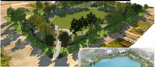
Dry detention basins/ dished landscaped areas which can be utilised for water storage in storm events. SW connection to existing stream/culvert in this area. Storm storage ponds near connection point are most beneficial from a SuDS perspective.
